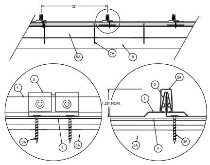
1. **Metal Roof Deck Panels\* -** No. 24 MSG min coated steel panels, 12 in. wide, 1-3/8 in. high at side ribs. Panels continuous over three or more clips with no endlaps. A bead of sealant may be used at panel side joints.
